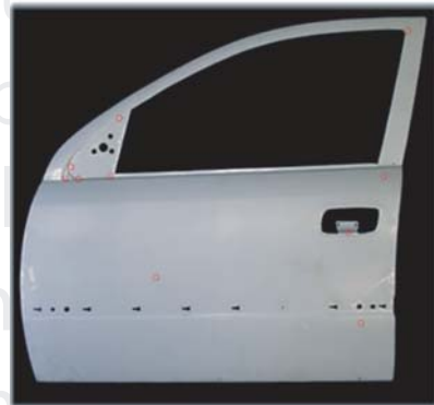
The strains are plotted on the forming limit diagram at different points across the surface can be calculated using circle grid analysis. In this example, all of the points on the FLD fall within the 'safe' area, and no failure (i.e. splitting or necking) is expected.
